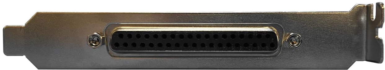
PCI/PCIe Card Connector CN1 (Black DB37)
